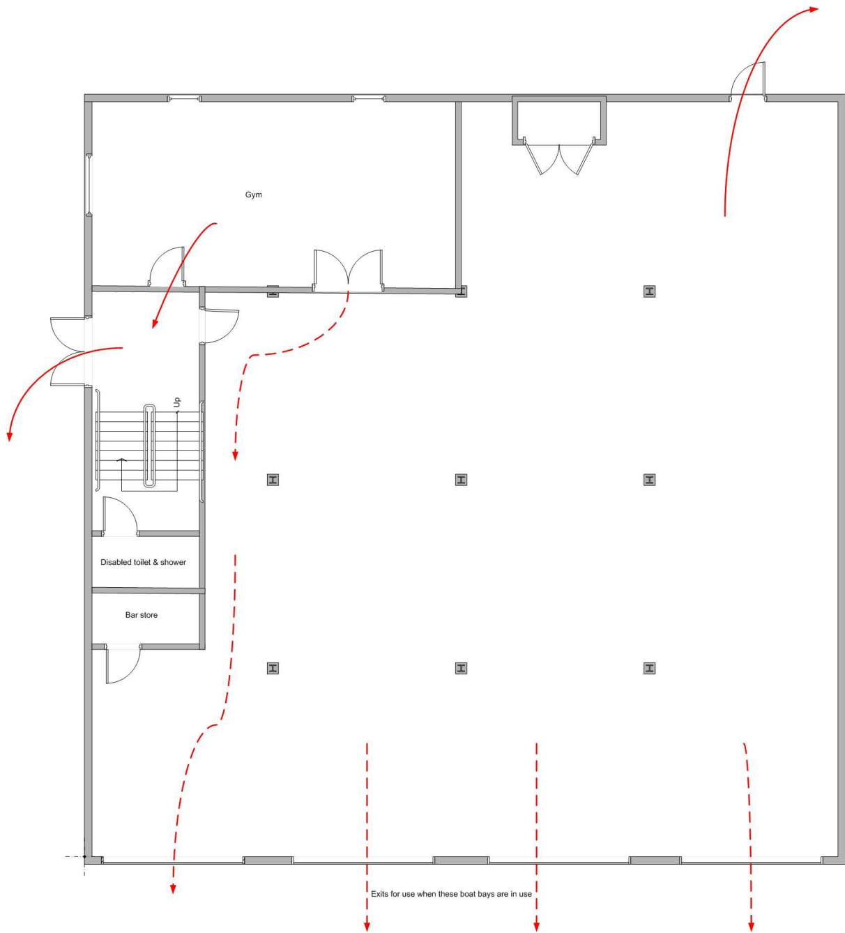
Figure 2 - Escape routes downstairs
